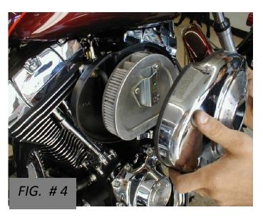
D. WITH ADAPTOR IN PLACE, LOCATE THE STOCK AIR BOX OVER THE ADAPTOR, UTILIZING THE STOCK AIR BOX GASKET (THERE SHOULD BE NO GAPS BETWEEN ADAPTOR, AIRBOX OR CARBURETOR WHEN PROPERLY INSTALLED) STAND-OFF SPACERS PROVIDED ARE TO BE PLACED BETWEEN AIR BOX & ENGINE HEADS BEFORE INSTALLING THE VENT/RETAINING BOLTS. FOR EVALUATION ENGINES STOCK VENT BOLTS CAN BE USED WITH LARGER I.D. SPACER PROVIDED.
